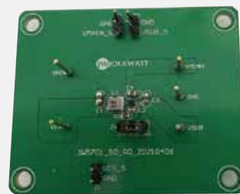
DC-DC Power Supply
