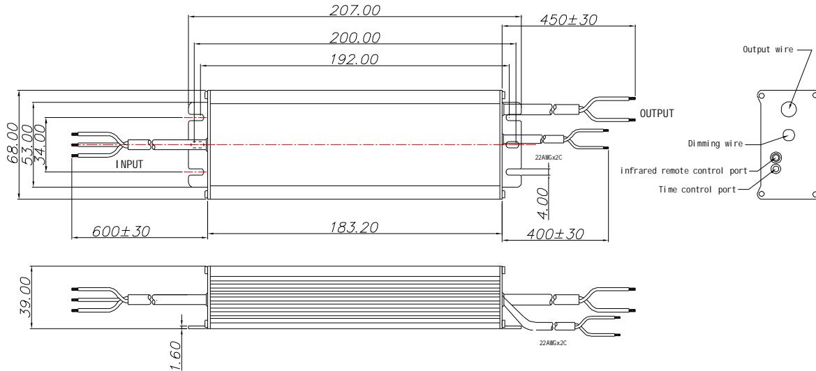
Note: Model LDP-150R214 no dimming wire.
